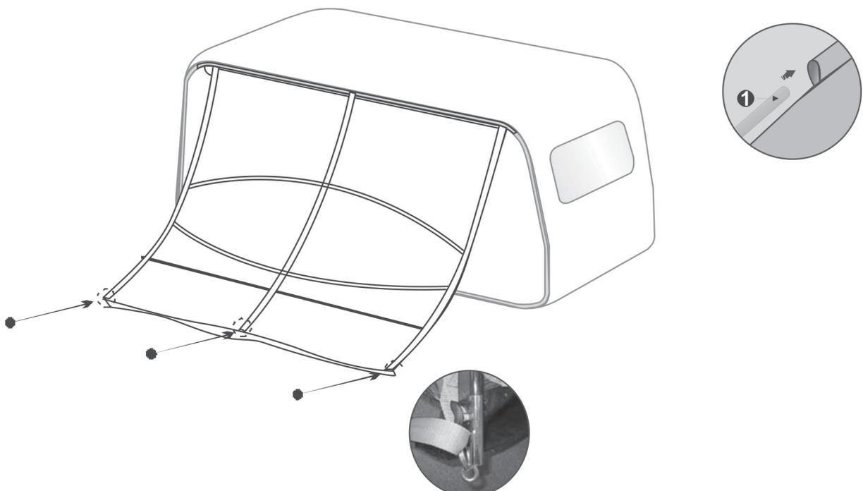
3. a) Assemble the roof pole 2 and make it tensioned.
