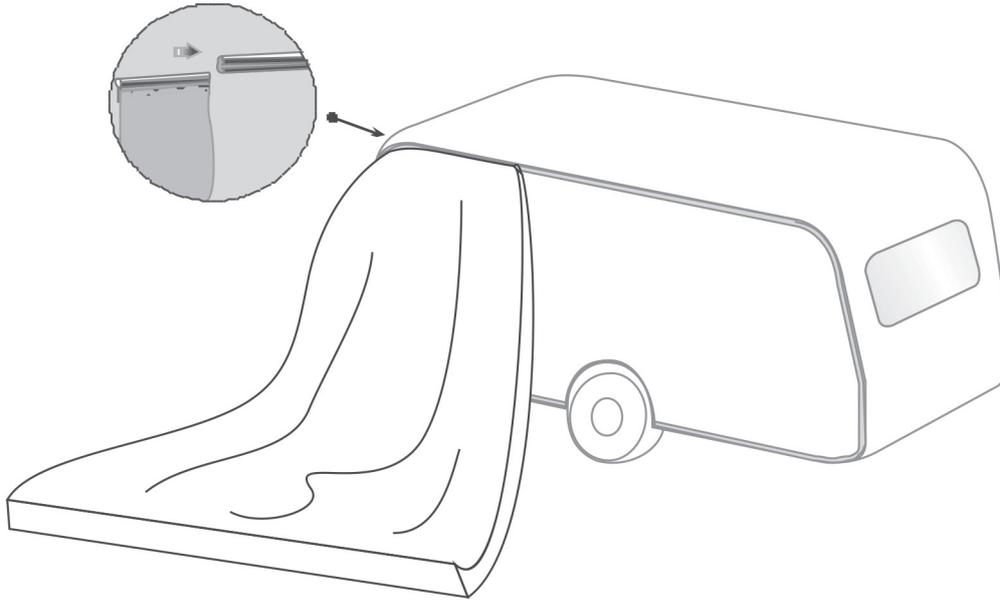
**2. a) Slide Pole 1 into the roof along the sleeve and fix the pole at bottom with a pin.**
